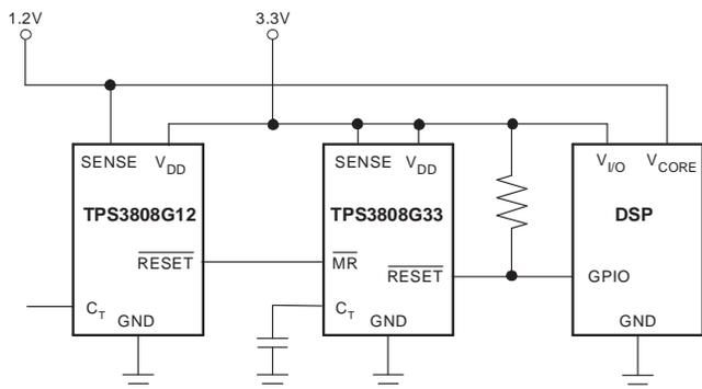
Figure 12. Using  $\overline{MR}$  to Monitor Multiple System Voltages
